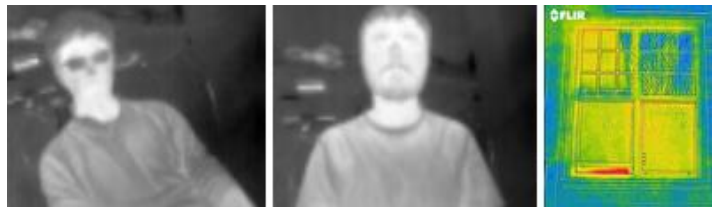
Figure 5: Corner cases include glasses, facial hair, and large warm windows in the background. (3)
